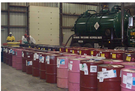
Figure 3. Container VAC liquid removal.
